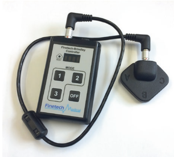
Fig. 2 External stimulator that can be programmed with different stimulation settings to enable the patient to stimulate for micturition, defecation, and erections separately. Signals are transmitted to the subcutaneous receiver block (Fig. 1) by the external stimulation block (Reprinted with permission of Finetech Medical Ltd.)
