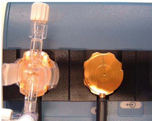
Figure 4.3 External fluid transducers. Left shown with disposable casing often called the 'dome' which is attached to the fluid containing tubing. Right shows the transducer without a 'dome'.
