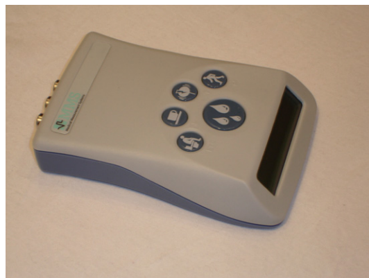
Figure 4.26 A modern Bluetooth portable ambulatory urodynamic device. Can be carried by the patient using a strap. The urodynamic catheters are attached to the connectors on the back of the device (just visible). The device also has event buttons for the patient to use.
