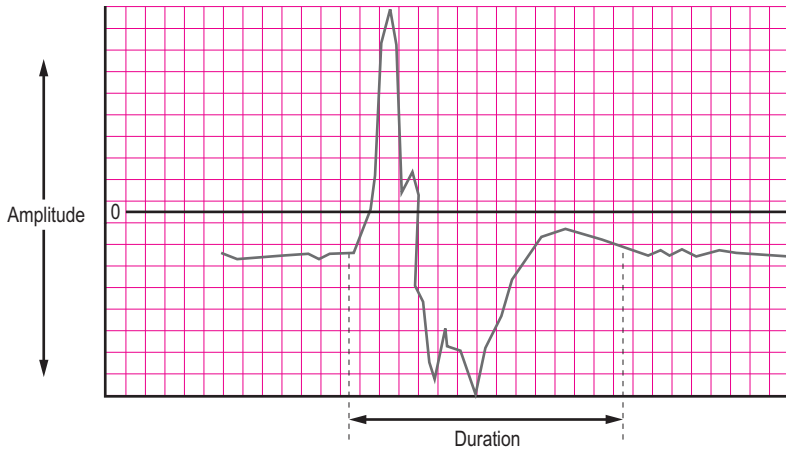
Figure 3.10 Muscle action potential from a urethral sphincter electromyogram.
